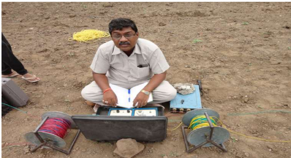
Photo 1 : Shows resistivity survey for subsurface rock identification
