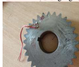
Fig.8.Bonding of strain gauge
