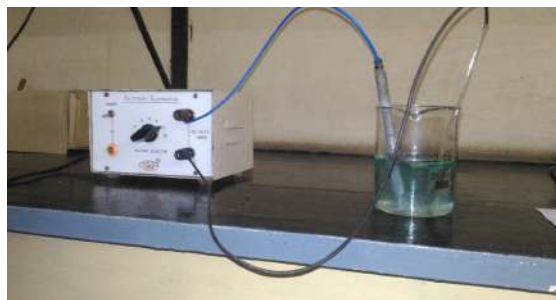
Figure 1: Experimental setup for electrolysis of copper sulphate
