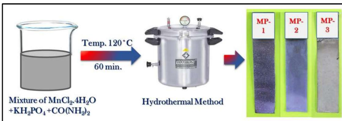
Scheme 1. The schematic diagram for preparation of manganese phosphate thin film using one-pot hydrothermal method.
